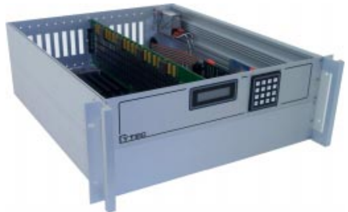
4600 Series Matrix w/one Switch Module Installed
